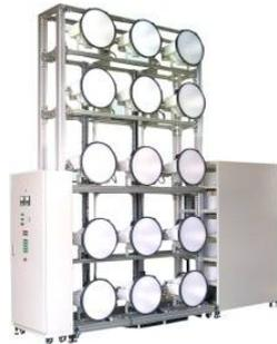
Solar simulator for PV module testing
